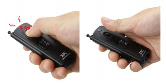
3. To release the shutter lock, press the shutter button of the transmitter again, the receiver will unlock the shutter. Then you will get plenty of pictures.
