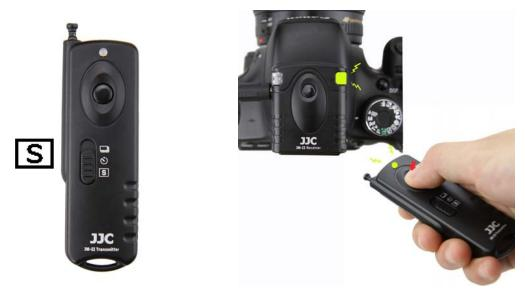
2. Then full press while holding the shutter button of transmitter until the transmitter LED light OFF, the receiver will now lock the shutter for continuous shot.
