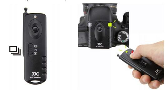
2. Then full press the shutter button, the camera will continuously take 3 pictures at an interval of 1s.
