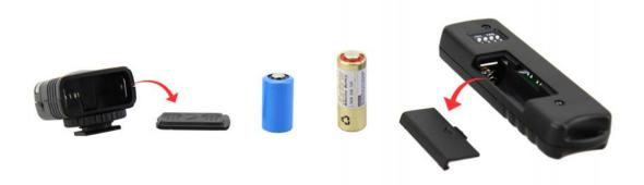
2. Insert the fresh battery, please ensure the batteries are put into a correct direction. Do not install batteries in the reverse direction as this could cause the batteries to leak corrosive liquids, generate heat or explode.
