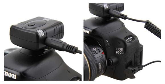
**Note:** Please remember not to connect the cable round the wrong way. For any JJC connecting cord, please always keep in mind that the end as the picture shown left should be plugged to receiver while the other end is for the camera remote socket.
