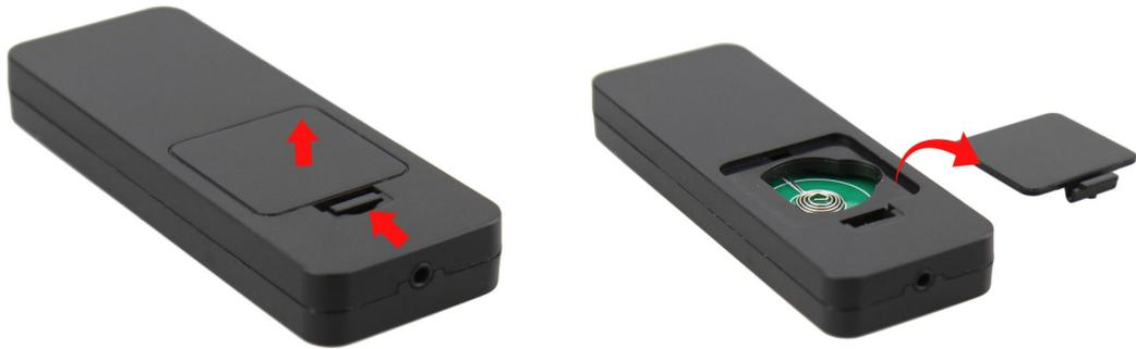
2. Insert a CR-2032 battery to the battery compartment with anode facing upwards and press down. Make sure battery is well installed into the battery compartment for use. Do not install batteries in the reverse direction as this could cause the batteries to leak corrosive liquids, generate heat or explode.
