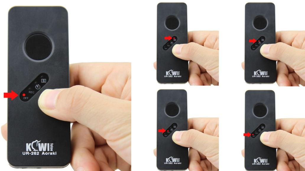
4. Then press the shutter button on UR-262 to enable the function you choose in step 3. When you press the shutter button of the UR-262, the specific function led light will flash.
